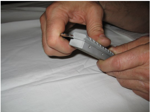
Pull out shift lever and turn to one side. Slide knife blade between top and bottom.
