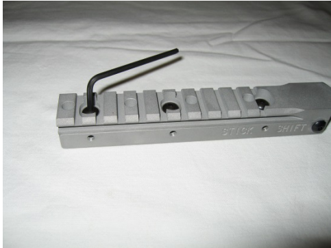
Remove three screws and nylon washers on top.
